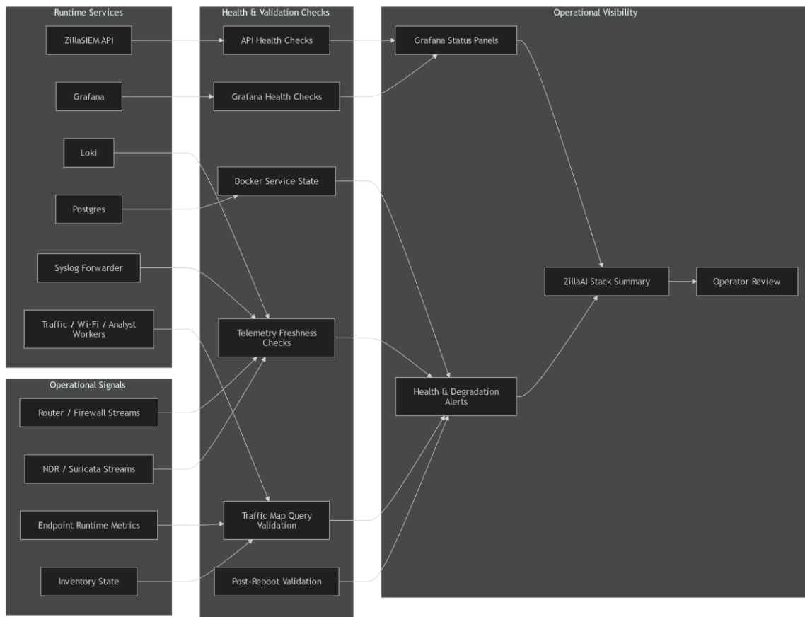
ZillaSIEM™ Operational Validation & Health Monitoring
